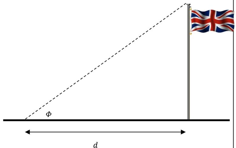
3.34 If the maximum error in  $d$  is, say, 0.1 m then the estimate of  $h$  could be anywhere between  $(7.0 - 0.1) \cdot \tan(37^\circ)$  m and  $(7.0 + 0.1) \cdot \tan(37^\circ)$  m, i.e., between 5.200 m and 5.350 m. So, a change of  $\pm 0.1$  m in the input quantity  $x_i$  has resulted in a change of  $\pm 0.075$  m in the output estimate  $y$ . The sensitivity coefficient is therefore estimated to be  $c_d = \frac{0.075}{0.1} = 0.75$ .
